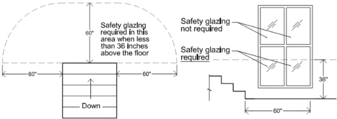
**7. Glazing Adjacent to Stairs and Ramps:** Glazing where the bottom edge is less than 36 inches above the plane of the adjacent walking surface of stairways, ramps, and landings between stair flights and ramp runs, must be safety glazing. (R308.4.6)
